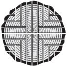
time, it is difficult, and you get several different board widths. Quarter sawing should not be applied when cutting small logs.
